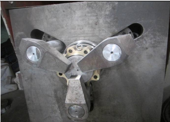
31 shell test of check valve
